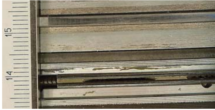
Fig. 6. View of the piston ring zone after engine running-in
